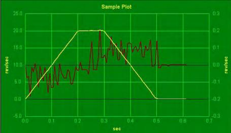
NOTE: When adjusting control loop gain values remember that the FF Term (KK) has no effect when operating in the Position – Pulse & Direction Control Mode.
