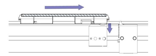
Figure 1: Pallet bumper conveys over antirebound stop, depressing the stop plate
